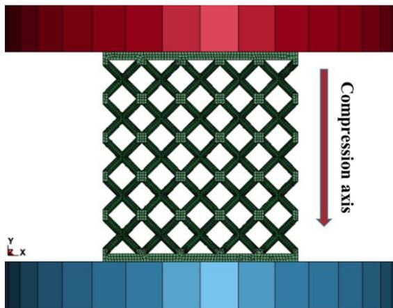
Figure 3. The compression test model of BCC lattice structure
