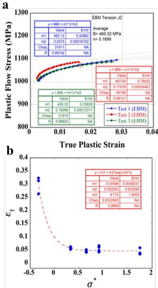
Figure 2. Determination of Johnson Cook parameters (a) A, B, n and (b)  $D_1$ ,  $D_2$   $D_3$  values
