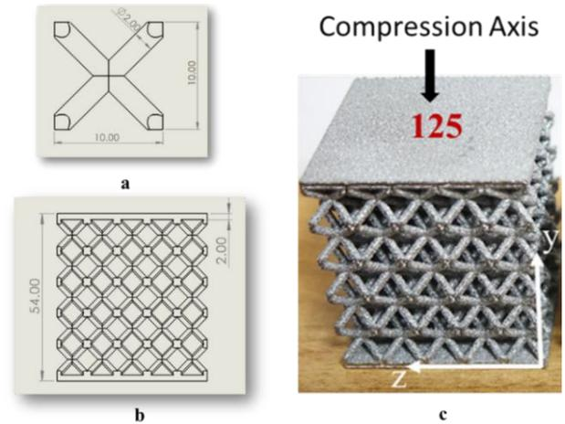
**Figure 1.** (a) CAD model of unit cell and (b) BCC Lattice Structure and (c) EBM-Ti64 BCC Lattice Structure
