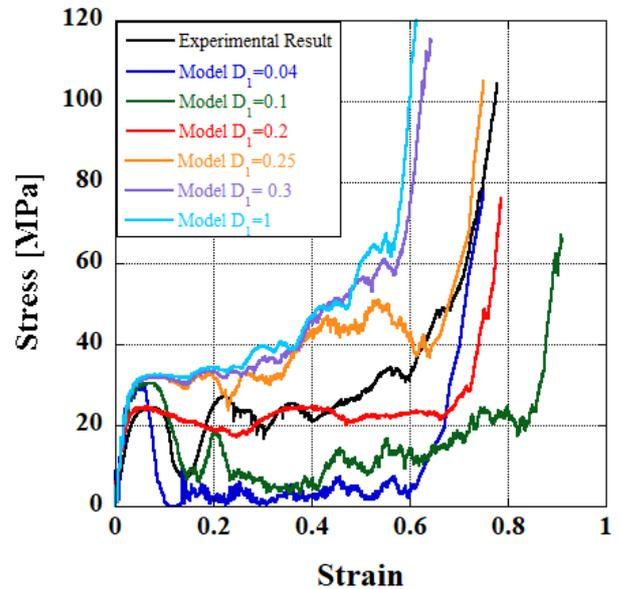
Figure 4. The stress-strain curves with different  $D_1$  parameter
