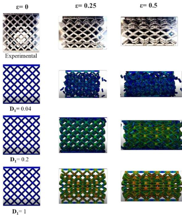
**Figure 5** The experimental numerical deformation stage of Ti64 BCC lattices at different strains and initial failure strain
